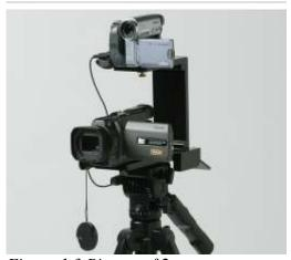
Figure 1.3 Picture of 2 cameras mounted on a Dual Stack Bar
